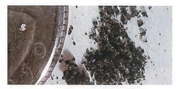
Black Particles inside a Plant Cartridge Filter (a quarter is shown in the image for scale)
